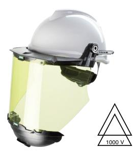
*V*-Gard **Electrician's Visors** provide reliable protection from arc flash effects: high temperature, flying debris and powerful radiation. They are certified to the highest European arc flash protection levels by the standards GS-ET-29 [class 2, 7 kA] and EN166 [8]. The impact and splash resistance is certified to EN 166 [B & 3].
